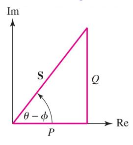
$\theta - \phi > 0$ : power factor is lagging (inductive load)
