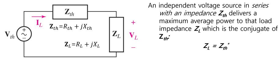
An independent voltage source in *series* with an impedance  $Z_{th}$  delivers a
