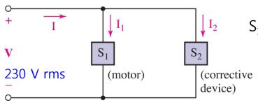
$S_1$ : 50 kW induction motor at a lagging PF of 0.8
