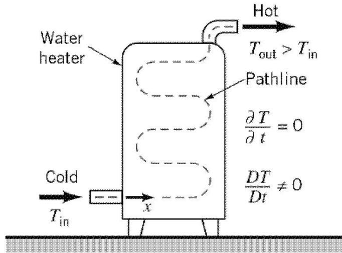
$$\frac{DT}{Dt} = \frac{\partial \vec{T}}{\partial t} + u \frac{\partial \vec{T}}{\partial x} + v \frac{\partial \vec{T}}{\partial y} + w \frac{\partial \vec{T}}{\partial z}$$
