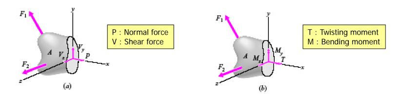
> Components of the internal force system can be found using the equilibrium equations
