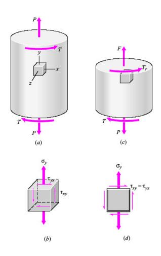
• Circular bar subjected to axial load P and torque T
