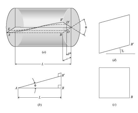
$\theta$ : angle of twist  $\gamma_{\rho}$ : shear strain at a distance  $\rho$  $\gamma_{c}$ : shear strain at a surface If the small strain is assumed
