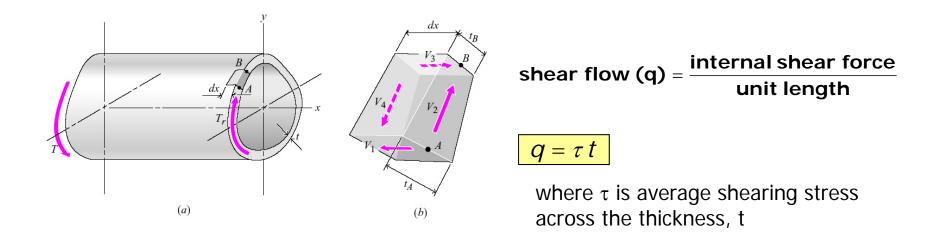
• Shear flow on the cross section is constant even though the wall thickness varies.
