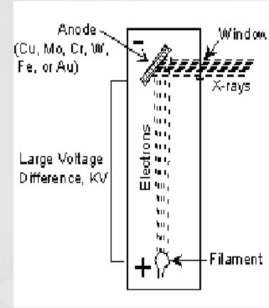
These electronic transitions results in the generation of X-rays. The X-rays then move through a window in the X-ray tube and can be used to provide information on the internal arrangement of atoms in crystals or the structure of internal body parts.
