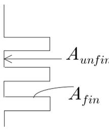
$$\begin{aligned} &= hA_{unfin}(T_b - T_\infty) + \eta_{fin}hA_{fin}(T_b - T_\infty) \\ \epsilon_{fin,overall} &= \frac{\dot{Q}_{total,fin}}{\dot{Q}_{total,nofin}} \end{aligned}$$
