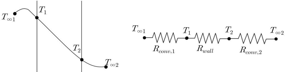
$$\begin{aligned} \dot{Q} &= \frac{T_{\infty 1} - T_{\infty 2}}{R_{conv,1} + R_{wall} + R_{conv,2}} = \frac{T_{\infty 1} - T_{\infty 2}}{R_{total}} \\ &= \frac{T_{\infty 1} - T_1}{1/h_1 A} = \frac{T_1 - T_2}{L/kA} = \frac{T_2 - T_{\infty 2}}{1/h_2 A} \end{aligned}$$
