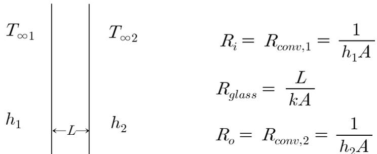
$$R_{total} = R_i + R_{glass} + R_o$$
