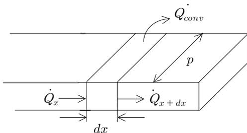
$$\dot{Q}_{cond,x} = \dot{Q}_{cond,x+\Delta x} + \frac{\dot{Q}_{conv}}{h(p\Delta x)(T-T_\infty)}$$
