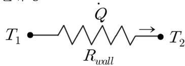
$$\dot{Q} = \frac{T_1 - T_2}{R_{wall}}$$
