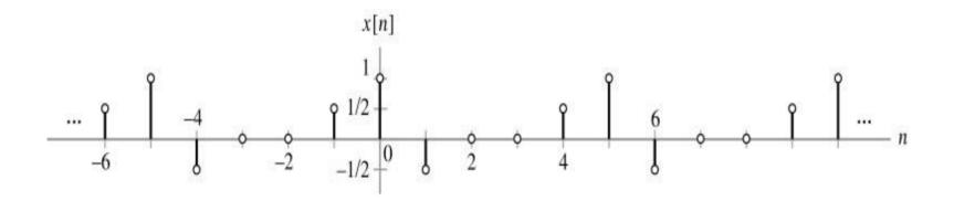
$$\begin{split} N &= 5; \qquad \Omega_0 = 2\pi/5; \qquad odd \qquad symmetry \\ X[k] &= \frac{1}{5} \sum_{n=-2}^{2} x[n] e^{-jk2\pi n/5} \\ &= \frac{1}{5} \left\{ x[-2] e^{jk4\pi/5} + x[-1] e^{jk2\pi/5} + x[0] e^{j0} + x[1] e^{jk2\pi/5} + x[2] e^{-jk4\pi/5} \right\} \\ &= \frac{1}{5} \left\{ \frac{1}{2} e^{jk2\pi/5} + 1 - \frac{1}{2} e^{jk2\pi/5} \right\} = \frac{1}{5} \left\{ 1 + j \sin(k2\pi/5) \right\} \end{split}$$
